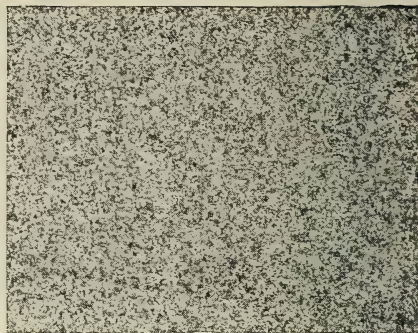
FIG. 123.—Prepared Roofing Finished with Coarse Talc.
